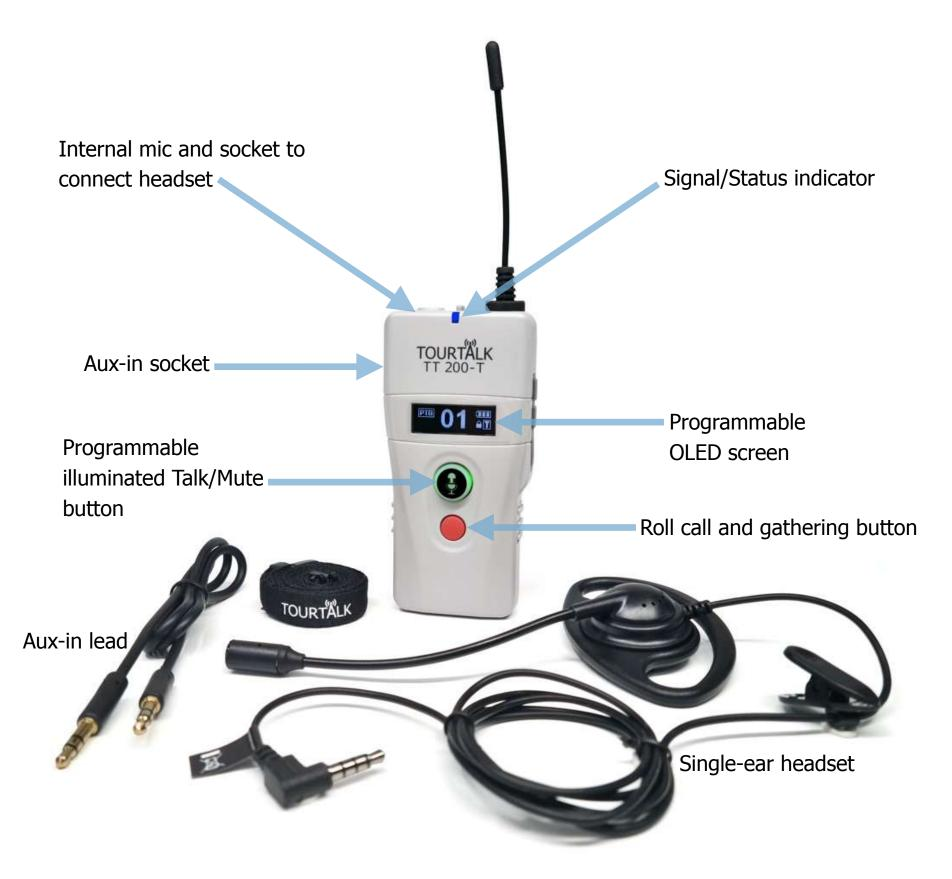
The digital Tourtalk TT 200-T is a transmitter and receiver in a compact, lightweight, simple to use unit enabling both one-way and two-way communication between group leaders and the tour group.
